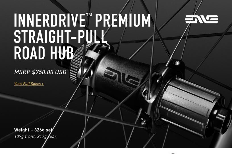
INNERDRIVE™ represents the pinnacle of bicycle drive mechanisms. Oversized steel ratchets are positioned inboard and over the bearings to reduce stress on the axle and bearings while ensuring positive, reliable engagement.
