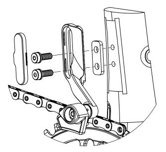
Note: the shim is flat on one side and curved on the other, the curved side should face the frame. Loosely tighten both bolts so you can still move the guide around.
