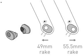
49mm rake / 140mm rotor
