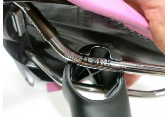
Apply very light coating of grease to each sliding wedge interface. Be very careful not to get grease on the bottom of the wedges that interface with the seat post barrel. This can cause saddle slipping issues.
