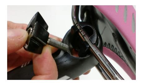
With you other hand, pick up the left side wedge and line it up with the bolt. Pinch assembly to hold it all in place.
