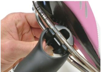
Slid in the right side wedge and bolt w/ greased surface interfacing with the lower rail cradle, and hold in place.
