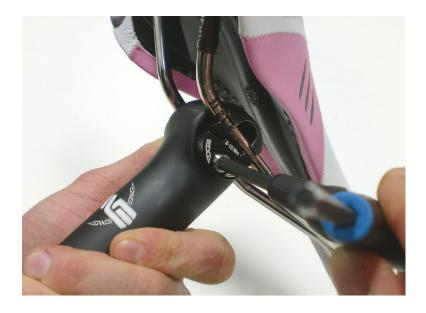
Once desired position is achieved, tighten bolt to 12nm.
