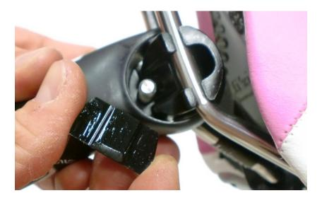
Use your 5mm Allen wrench to tighten the bolt until the clamp assembly is compressed. Leave assembly loose enough to saddle angle and position.
